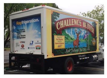
is also capable of charging the battery while the vehicle is running. Challenge Dairy has been testing the Rayfridgeration truck since April 2017, and it is exceeding expectations so far. As compared to a conventional refrigerated delivery truck, the Rayfridgeration truck has reduced nitrous oxide emissions by 98%, carbon dioxide emissions by 86%, and particulate matter emissions by 97%.
